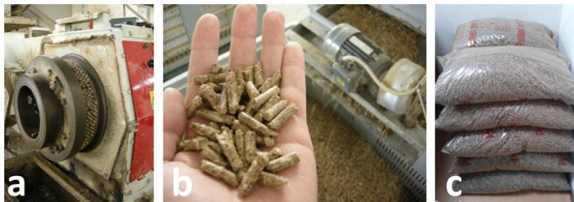
Fig. 2. Schematic of the pelletization process showing (a) pellet mill,(b) Olive and Hazelntu's pellet and (c) packaging.
