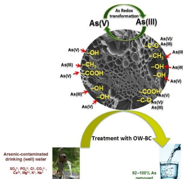
Fig. 2. Sorption of As onto the surface of BC, a general mechanism, adopted from Khan et al., (2018)[120].
