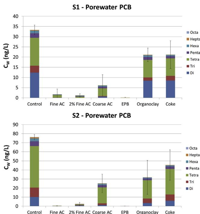
**Fig. 1.** Reductions in PCB homolog porewater concentrations in S1 and S2. All amendments were added at a 5% dry weight dose, except for the 2% fine AC. Error bars represent standard deviations ( $n = 3$ ).
