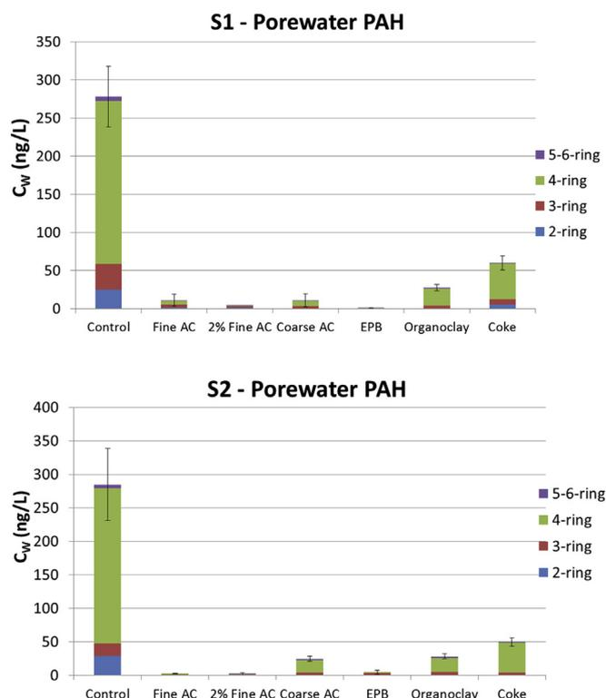
**Fig. 2.** Reductions in PAH porewater concentrations in S1 and S2. All amendments were added at a 5% dry weight dose, except for the 2% fine AC. Error bars represent standard deviations ( $n = 3$ ).
