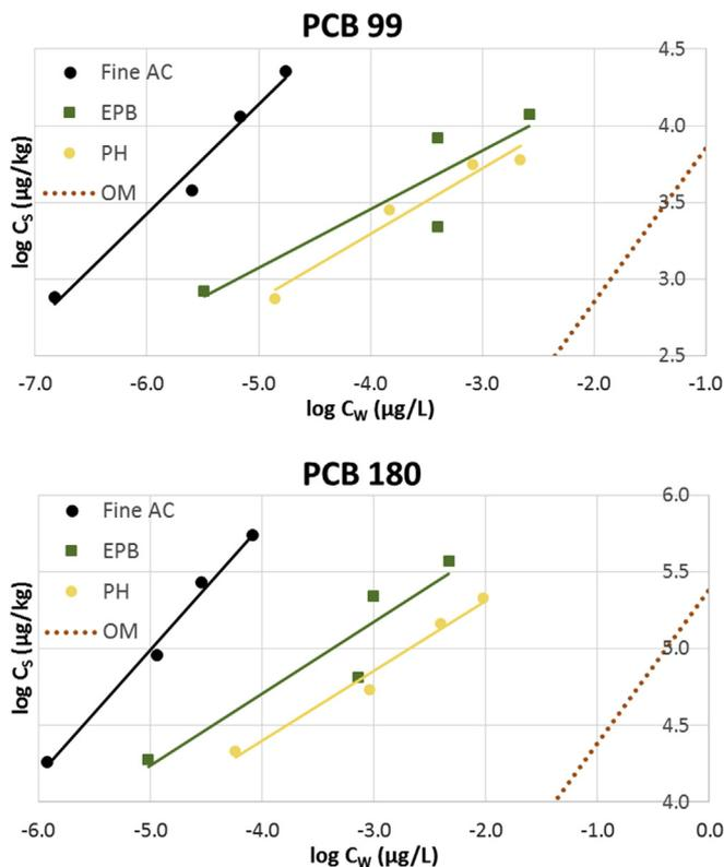
Fig. 5. Sorption isotherms for PCB congeners 99 and 180 plotted using data presented in Table S7 for fine AC and biochar. PH is a peanut hull biochar that was found to be amongst the most sorptive biochars in a previous study (Gomez-Eyles et al., 2013a, b). A dotted brown line is used for the predicted sorption to natural organic matter (OM) (LaGrega et al., 1994). (For interpretation of the references to colour in this figure legend, the reader is referred to the Web version of this article.)
