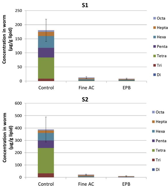
Fig. 3. Reductions in total PCB bioaccumulation in S1 and S2. Error bars represent standard deviations ( $n = 4$ ).
