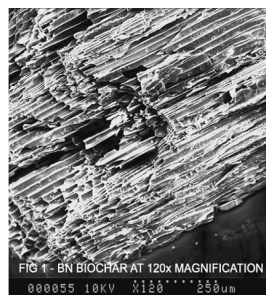
BioChar at 120x & 1,200x Magnification
